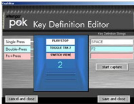
Fig. 5 (click to enlarge): The Key Definition Editor is where you program the individual footswitches. To edit an individual switch, you click on it. This opens up the Key Definition Editor, which will look something like the shot to the left.
